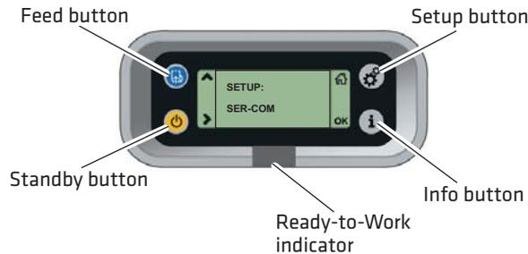
**Printer Control Panel:** Use this illustration to familiarize yourself with the buttons and lights on the printer.
