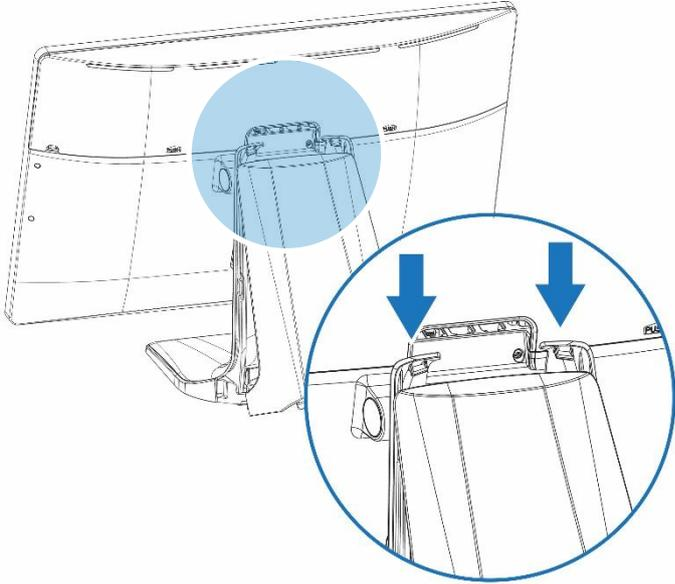
Step5. Assemble upper and push the bottom.
