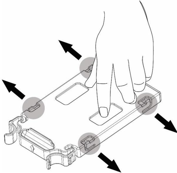
Step3. Remove SSD or HDD by pushing four hinges on the side as below.
