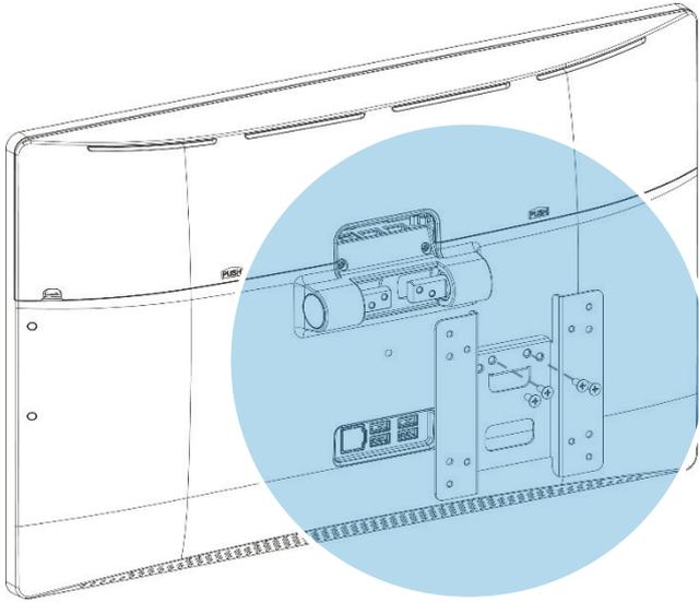
Step3. Assemble "Vesa bracket(A)" with the screws(E).
