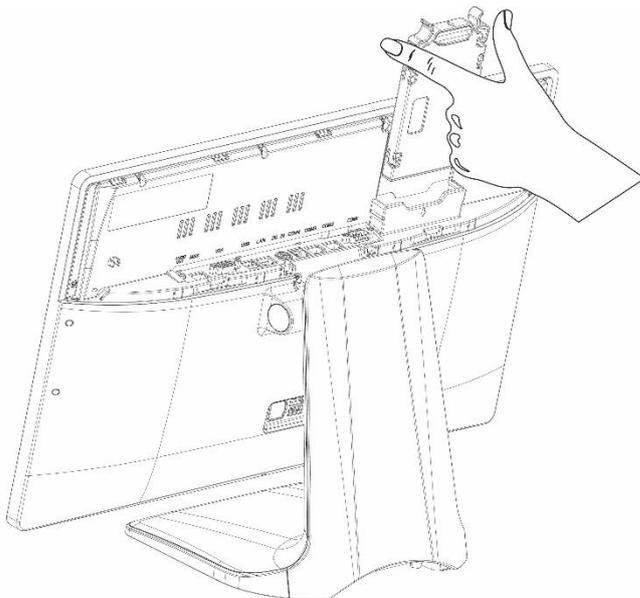
Step3. Pull the HDD Tray handle and
