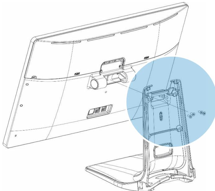
Step2. Separate four screws (E).
