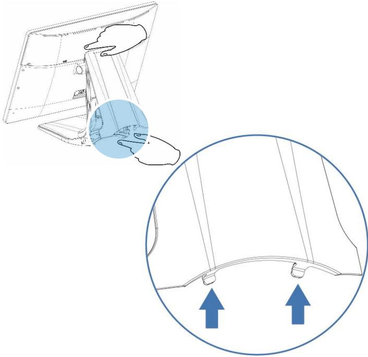
Step1. Separate it while holding the product of the handle & pulling the bottom hook of "stand cover".
