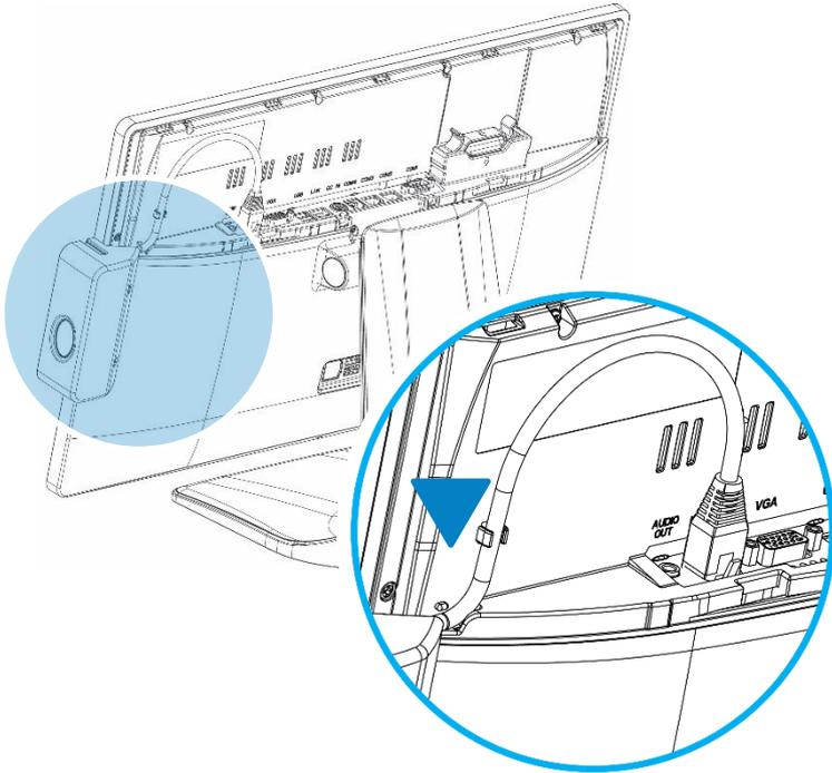
Step4. Connect the cable to MSR port.
