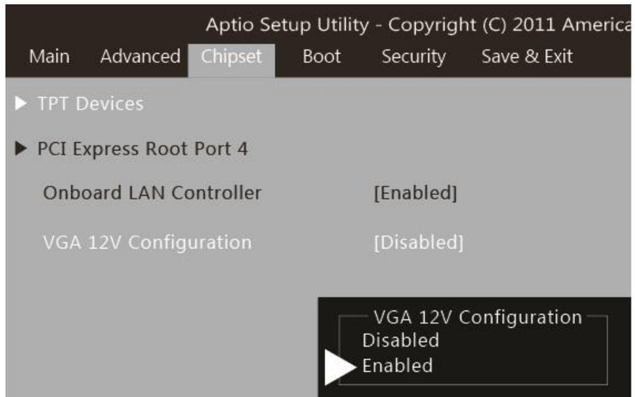
Step6. Change VGA 12V Configuration - Disabled to Enabled.
