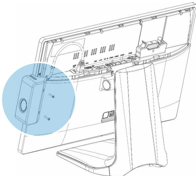
Step3 Fix the MSR Module using screws
