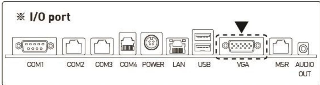
Step4. Connect the cable of 2nd display after refer to the image.
