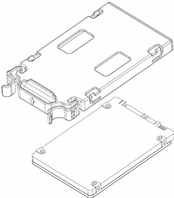
Step4. Secure SSD or HDD to the bottom of the tray with the sticker facing outward.
